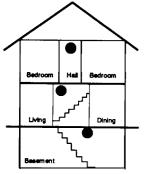
A Smoke Detector should be located on each story.
